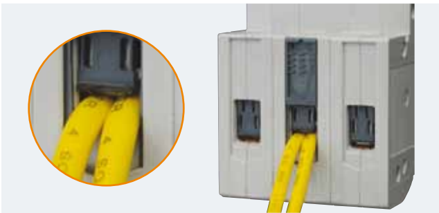
Terminals can accommodate 2 wires of same cross section (Solid up to 2 X 10 mm 2 and finely stranded with end sleeve up to 2 X 4 mm 2 ) without twisting wire strands facilitates easier and safe wiring
